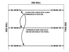
4. Hang up your net by attaching the net's thick Polypropylene rope to the cables by means of snap rings. Rings should be 18" apart.
