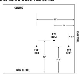
3. Attach the cables as follows: OVERHEAD VIEW
