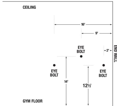
**3. Attach the cables as follows: OVERHEAD VIEW**
