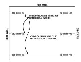
**4.** Hang up your net by attaching the net's thick Poly-Dac rope to the cables by means of snap rings. Rings should be 18" apart.
