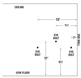
$oldsymbol{3}_{oldsymbol{\cdot}}$  Attach the cables as follows: <code>OVERHEAD</code> <code>VIEW</code>
