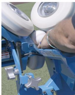
**NOTE:** When feeding balls into the mini3™ for fly balls, ball should be entered into the ball chute, resting on back of fingers, and "flicked" into the tires.
