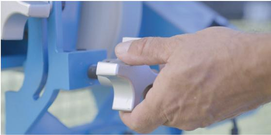
*Figure 6. Vertical Micro-Adjustment Knob.*
