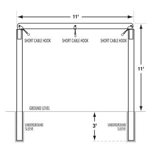
2. Once you assemble them, the three middle sections will look like this. On all three insert a short hanging-loop assembly into the middle pre-drilled crossbar hole and long hanging-loop assemblies into both outside pre-drilled crossbar holes.
