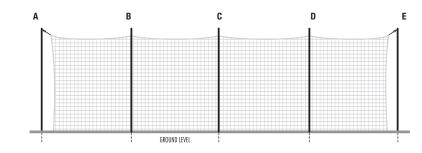
Ropes attach to the hanging-loop assemblies on crossbars A, B, C, D, and E.
