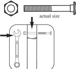
Join the frame sections. Fasten together, using nuts, and short carriage bolts. tighten nuts with the supplied wrench.
