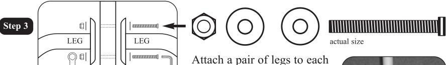
end of the frame, using nuts, washers and <u>long</u> bolts.
