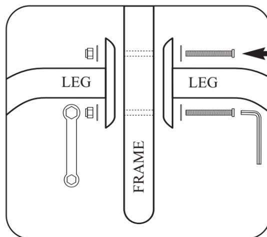
Attach a pair of legs to each end of the frame, using nuts, washers and long bolts. Tighten bolts with the Allen wrench (shown in drawing).
