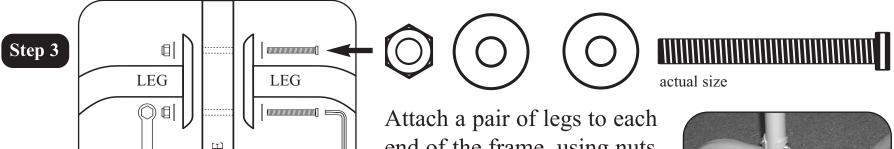
Attach a pair of legs to each end of the frame, using nuts, washers and <u>long</u> bolts.
