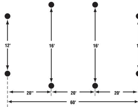
**4.** SIDE VIEW OF THE FOUR U-SHAPED SECTIONS COMPLETELY SET UP.
