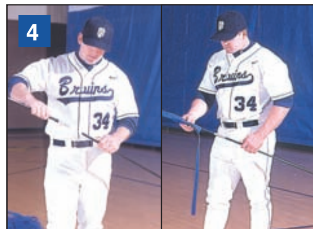
4. Put folding Support Pole together at its maximum length of 25 feet. Slide blue Slipcover over assembled folding Support Pole .
